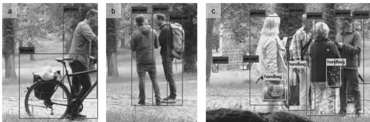
Figure: Bounding boxes around classified objects detected by YOLO
